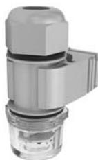
Photosensor SKS-200 is external and is connected to terminals T1. Sensor is installable to panel (by screw-able transparent cover) to opening with diameter 20 mm. A part of the sensor is a plastic holder for placing into the wall or to another place. Length of a line connector to the sensor cannot be more than 50 m. Double-core cable can be used as wire diameter min. 0.2 - 0.75 mm<sup>2</sup> / with sleeve: 0.25 - 0.34 mm<sup>2</sup>.
