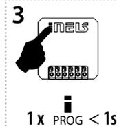
Press of programming button on actuator RFSAI-61B-SL shorter than 1 second will finish programming mode, LED switches off.
