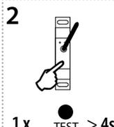
Press and hold the TEST button on RFSG-1M for more than 4s to automatically assign the RFSG-1M transmitter to the actuator.
