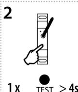
Press and hold the TEST button on RFSG-1M for more than 4s to automatically assign the RFSG-1M transmitter to the actuator.
