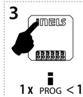
Press of programming button on actuator RFSAI-61B-SL shorter than 1 second will finish programming mode, LED switches off.
