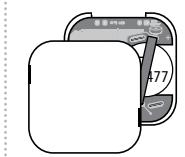
After finished programming, insert the device into the box and snap on the rear cover.
