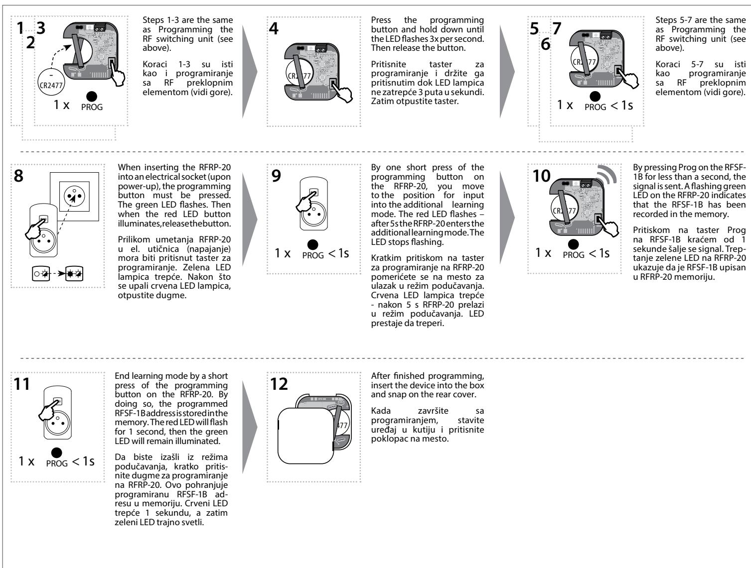
Programming with the RF control unit RF Touch / Programiranje sa RF sistemskim elementom RF Touch
