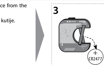
Remove the old battery from the battery holder.
