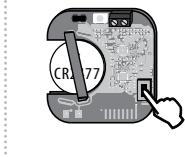
Press the programming button and hold down until the LED flashes once per second. Then release the button.
