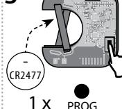
While pressing Prog on the RFSF-1B, insert the battery. Observe the polarity. This activates the programming mode. The red LED flashes in an interval of 2 flashes per second. After inserting the battery, release the button.
