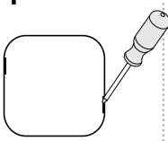
Using a screwdriver, carefully remove the rear cover.
