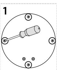
Use a screwdriver to open the detector.
