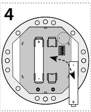
Insert / remove the battery into the detector according to the required function, ie: 1x battery insertion / removal - function 1, 2x battery insertion / removal - function 2... Each insertion must be signaled by flashing blue LEDs, there must be a delay of 1s between individual inserts.
