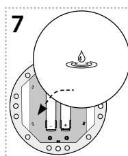
Replace the seal, attach the front cover - make sure the correct location. Screw in, tighten the screws to maintain IP protection.
