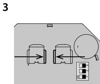
Before installing, open the detector cover with a screwdriver (Fig. 1). The adjustment settings are located inside the detector. Remove the insulating foil, check the correct placement of the battery.
