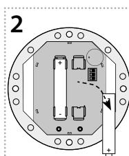
Remove one of the batteries from the holders.
