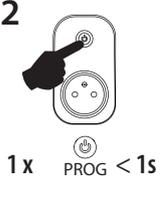
Pressing the programming button on the RFSC-61N receiver for less than 1 second will finish the programming mode, this will reverse the memory function. The LED lights up according to the current pre-set memory function. The set memory function is saved. Every other change is made in the same way.
