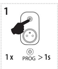
Press of programming button on receiver RFSC-61N for 1 second will activate receiver RFSC-61N into programming mode. Red LED is flashing in 1s interval.
