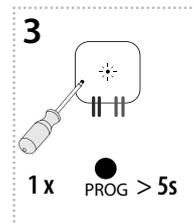
Press of programming button longer than 5 seconds, will activate actuator into timing mode. LED flashes 2x in each 1s interval. Upon releasing the button, the delayed return time starts counting.
