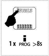
By pressing the programming button on the actuator for 8 seconds (RFSAI-61B-SL: press for 5 second), deletion of one transmitter activates. LED flashes 4x in each 1s interval. Pressing the required button on the transmitter deletes it from the actuator's memory. To confirm deletion, the LED will confirm with a flash long and the component returns to the operating mode. The memory status is not indicated. Deletion does not affect the pre-set memory function.
