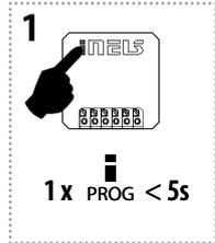
Press of programming button on receiver RFSAI-62B for 3-5 s (RFSAI-61B-SL: press for more than 1s) will activate receiver RFSAI-62B into programming mode. LED is flashing in 1s interval.
