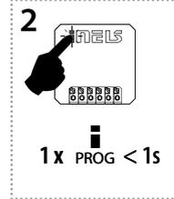
Pressing the programming button on the RFSAI-62B receiver for less than 1 second will finish the programming mode, this will reverse the memory function. The LED lights up according to the current pre-set memory function. The set memory function is saved. Every other change is made in the same way.
