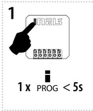
Press of programming button on receiver RFSAI-62B for 3-5 s (RFSAI-61B-SL; press for more than 1 s) will activate receiver RFSAI-62B into programming mode. LED is flashing in 1s interval.
