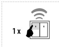
The output contact will be closed by pressing the button and opened after the set time interval has elapsed.
