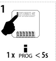
Press of programming button on receiver RFSAI-62B for 3-5 s (RFSAI-11B-SL: press for more than 1s) will activate receiver RFSAI-62B into programming mode. LED is flashing in 1s interval.
