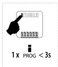
Channel selection (RFSAI-62B-SL) is done by pressing the PROG buttons for 1-3s. RFSAI-61B-SL: press for more than 1 second. After button release, LED is flashing indicating the output channel: red (1) or green (2). All other signals are indicated by corresponding color of LED for each channel.
