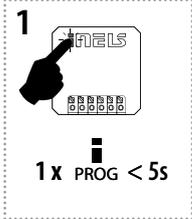
Press of programming button on receiver RFSAI-62B for 3-5 seconds (RFSAI-61B-SL: press for 1 second) will activate receiver RFSAI-62B into programming mode. LED is flashing in 1s interval.
