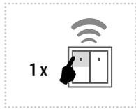
The output contact will be closed by pressing the button and opened by releasing the button.
