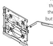
After removing the control flaps, the programming button is accessible.
