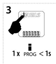
Press of programming button on receiver RFSAI-62B shorter than 1 second will finish programming mode. The LED lights up according to the pre-set memory function.
