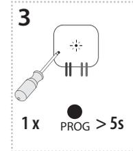
Press of programming button longer then 5 seconds, will activate actuator into timing mode. LED flashes 2x in each 1s interval. Upon releasing the button, the delayed return time starts counting.
