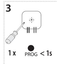
Press of programming button on receiver RFSA-62B shorter than 1 second will finish programming mode. The LED lights up according to the pre-set memory function.
