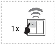
The output contact will be closed by pressing the button and opened by releasing the button. For the correct execution of individual commands (press = closing / releasing the button = opening), the time delay between these commands must be a min of 1s (press - delay 1s - release).
