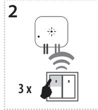
Three presses of your selected button on the RF transmitter assigns the function switch off (must be a lapse of 1s between individual presses).
