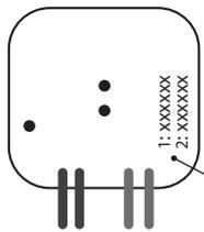
addresses for individual relays (channels) / adresy pro jednotlivá relé (kanály)
