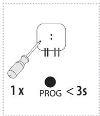
Channel selection is done by pressing the PROG buttons for 1-3s. After button release, LED is flashing indicating the output channel: red (1) or green (2). All other signals are indicated by corresponding color of LED for each channel.
