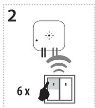
Assignment of the delayed on function is performed by six presses of the selected button on the RF transmitter (must be a lapse of 1s between individual presses).
