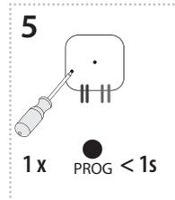
Press of programming button on receiver RFSA-62B shorter then 1 second will finish programming mode. The LED lights up according to the preset memory function.
