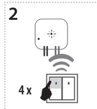
Four presses of your selected button on the RF transmitter assigns the function impulse relay (must be a lapse of 1s between individual presses).
