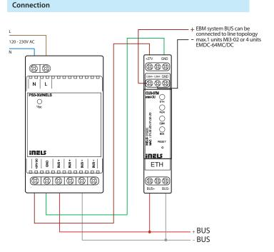
max. 32 units per BUS; max. 1A (PS3-30 / iNELS) per BUS
