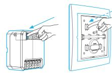
To clear an already paired channel to a button on the controller, press the PROG on the device for a period of time of 5 s or 7 s (see, **Tab 1**). Clear the memory of the button and press the appropriate button on the controller that you want to unpair. After this step, it returns to its working state.
