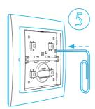
Short press (>1s) of the pairing button to exit the pairing mode
