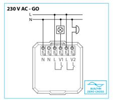
Output contact V1 is at the same potential as the product power supply. Output contact V2 is separate from the power supply but must be connected to the same potential. The wiring is used when it is necessary to secure V1 and V2 separately.
