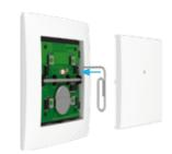
By removing the controller flap, the pairing button is accessed.
