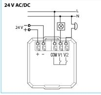
The output contacts (V1, V2) are galvanically isolated from the power supply and share a common COM
