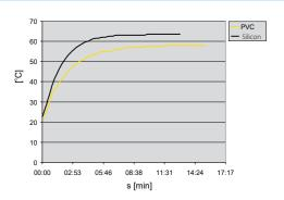
PVC -reaction to water temperature from 22.5 °C to 58 °C. Silicone - reaction to water temperature from 22.5 °C to 63.5 °C.
