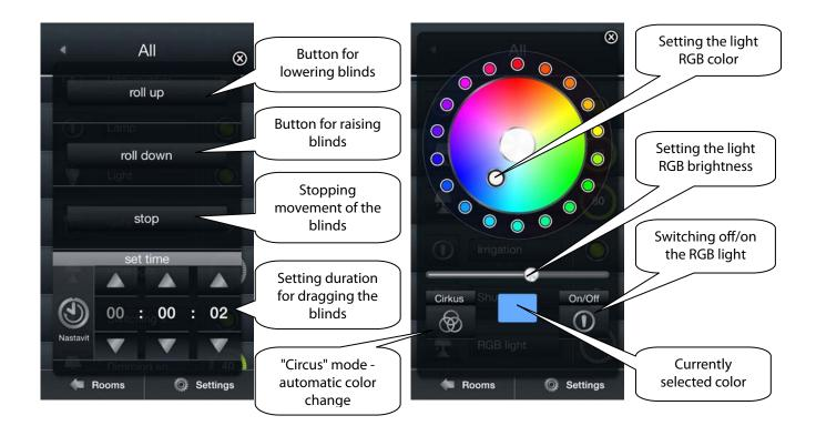
By pressing and holding the RGB actuator, you will see the menu displayed for setting color, brightness and the brightening mode.
