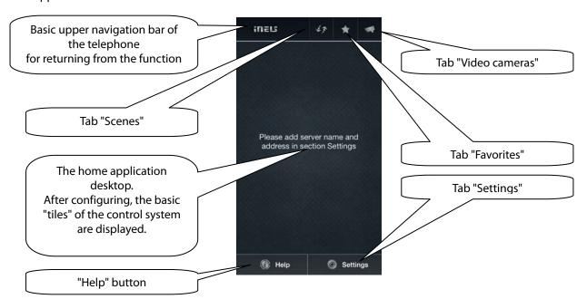
The aim when using the application for controlling the installation is so that after restarting it, it immediately offers control of the electrical installation. To achieve this with the least amount of presses and so that everything required would be offered right from the home desktop, you must first set up and configure the application.
