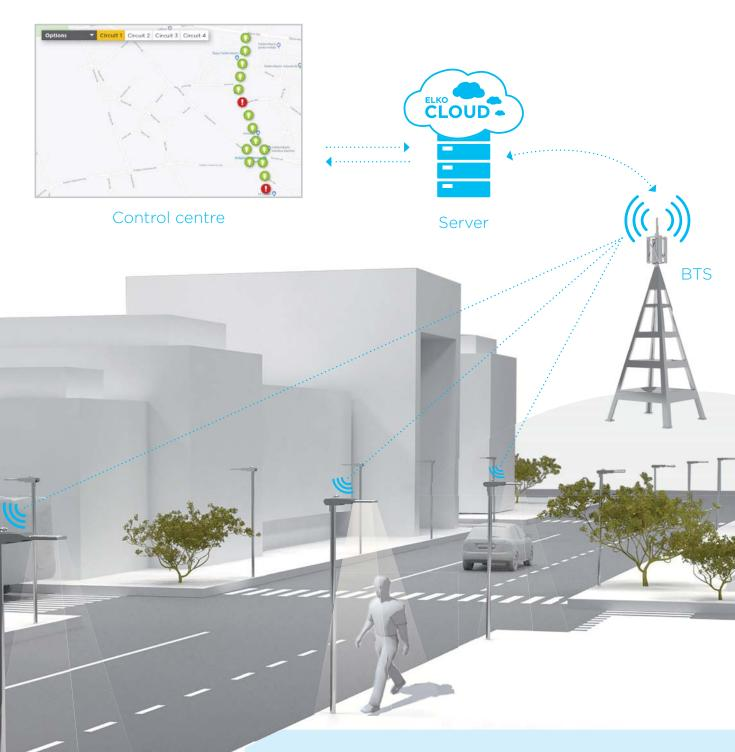
The main component of the infrastructure is the LoRA/NB-IoT LPWAN network that provides connectivity for IoT devices in Smart City.
