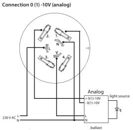
Description of wiring contacts: 1.0(1) - 10 V (-) 2.0(1)-10 V (+) 3. not connected 4. not connected L (LINE)- phase N (NEUT) - neutral V (LOAD) - switched output
