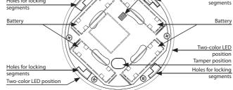
The underside of the detector
