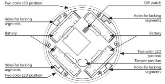
The underside of the detecto
