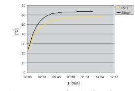
PVC -reaction to water temperature from 22.5 1°C to 58°C. Silicone - reaction to water temperature from 22.5°C to 63.5°C. **Accessories**
