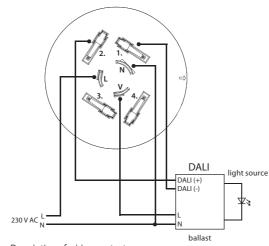
Description of wiring contacts: 1. DALI -2. DALI + 3. not connected 4. not connected L (LINE)- phase N (NEUT) - neutral V (LOAD) - switched output
