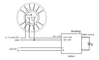
In the off state, the analog ballast may light up slightly (depending on gear type.
