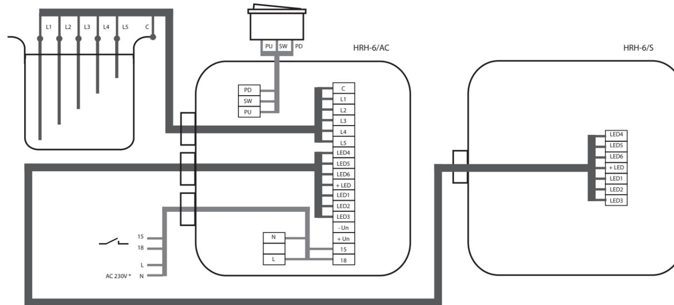
\* In case of HRH-6/DC, incoming supply is connected on terminals +Un and - Un.
