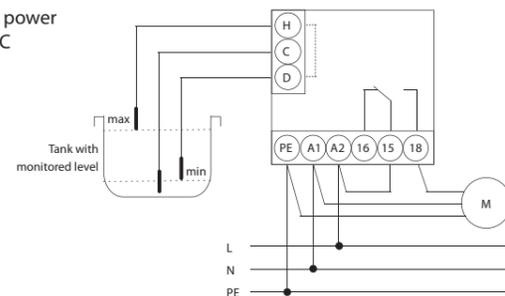
connection for power supply 24.. 240 V AC/DC
