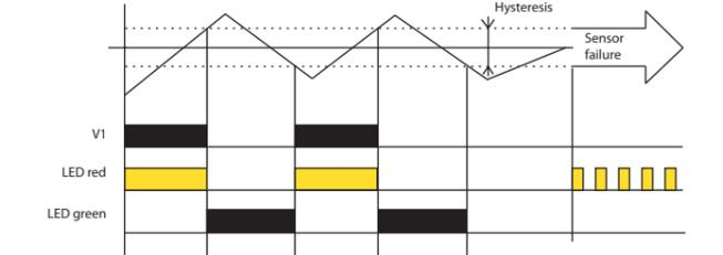
TEV-2 and TEV-3 are universal single thermostats for universal use. In case ambient temperature is higher than set temperature relay is open (function HEATING), for cooling function (opposite function) is possible to use NC contact of relay (V2).
