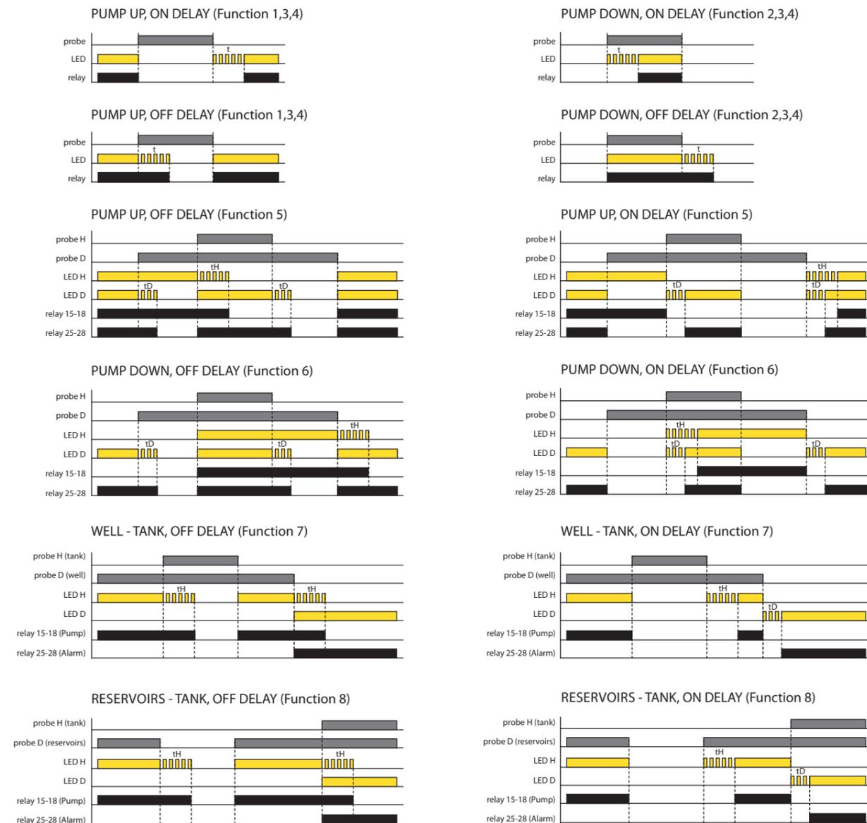
The relay is designed to monitor the level of conductive liquids with a choice of 8 functions:
