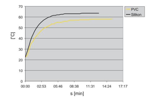
PVC -reaction to water temperature from 22.5 1 °C to 58 °C (from 72.5 °F to 136.4 °F).
