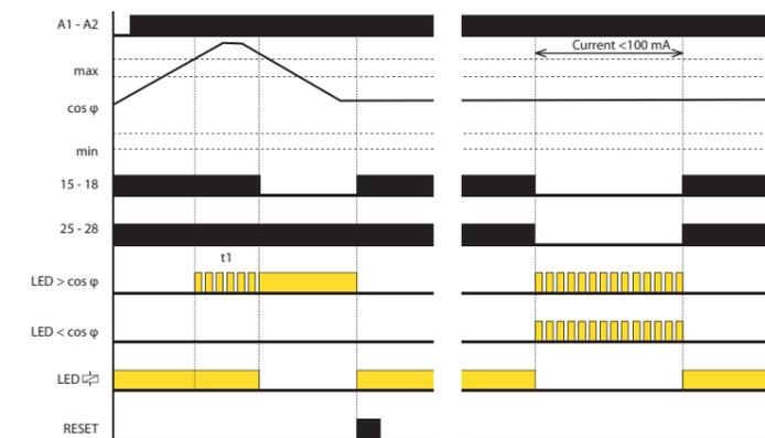
After powering on, the device sets the delay time t1 and yellow LED flashes. Both relays are switched on. The delay serves to eliminate a faulty state when starting the motor. After the time delay t1 begins monitoring COS φ only.
