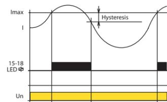
Monitoring relay PRI-32 serves to monitor current level in single phase AC circuits. Due to its fluent adjustment of release current, it is predestined for applications with necessity of current flow indication, and can be used as precedence relay. Output relay is off in normal state. In case the set current level is exceeded, it switches. Multivoltage supply is an advantage.
