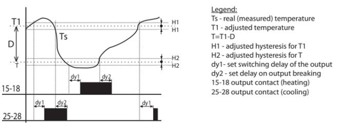
Classic function of thermostat, output contact switched until adjusted temperature is reached. Hysteresis eliminates frequent switching - output oscillation.
