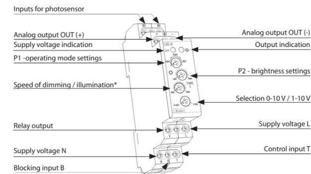
\* if the level of brightness on P2 is set on maximum the range is 24...120s
