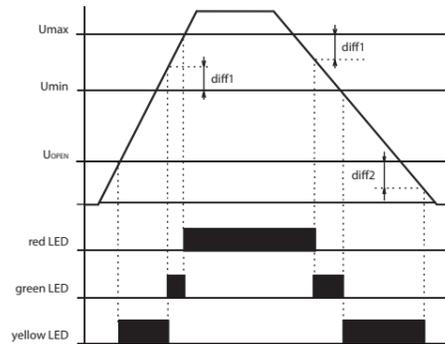
After connecting the supply voltage, the LED illuminates - the color corresponds to the voltage size of individual phases. If the phase voltage drops under 40 V (phase outage), the corresponding LED is not illuminated.
