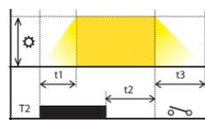
The switch starts the cycle and it stops on max.set brightness. After the switch is off, the cycle will continue until completed.
