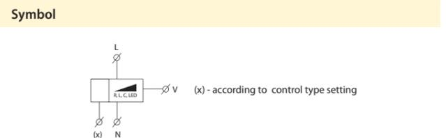
\* Warning: it is not allowed to connect inductive and capacitive loads at the same time.
