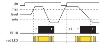
An AC current is used for measuring to prevent polarization and electrolysis of fluid and unwanted oxidation of measuring probes. Three probes are used for measuring: H - upper level, D - lower level and C - common probe. If using a tank made from conductive material, it is possible to use the tank itself as probe C. If it is necessary to monitor only one level, there are two connection options:
