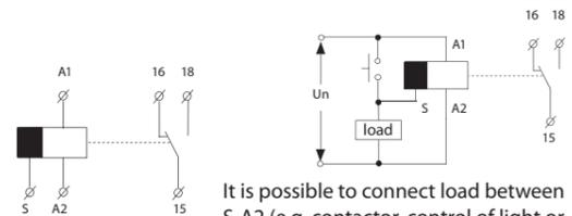
It is possible to connect load between S-A2 (e.g. contactor, control of light or any other device), without disturbing a correct function of relay (load is energized while the switch is ON).
