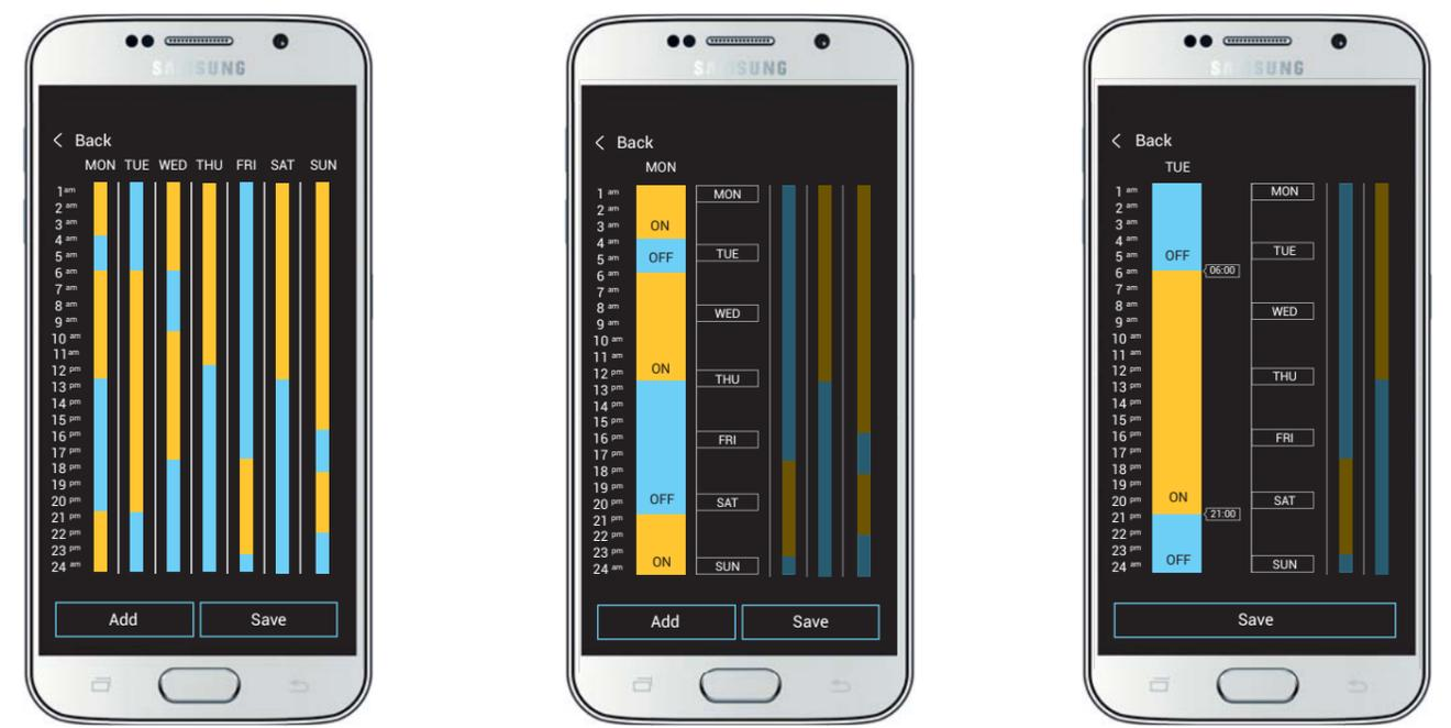
Through simple steps in the application you can set the desired on and off settings based on real time. You can copy this setting to other days, and altogether you can store up to 100 programs. The entire setup project can be saved to your smartphone and transferred to the next timer switch. The smartphone application serves not only to upload settings but also to download. The main benefit is speed and simplicity.
